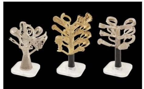
Direct casting using DigitalWax resins
